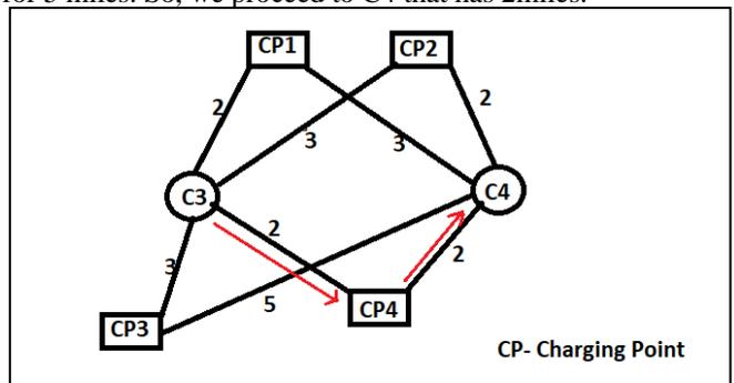
Fig 2: Finding the shortest path between delivery points via charging points.
